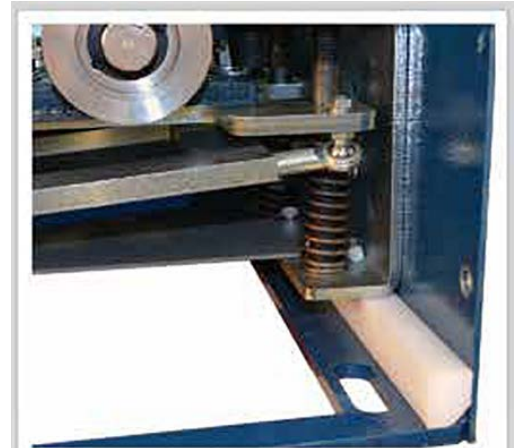
Spring mounted suspension that moves with rail
